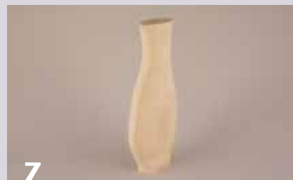
7 The workpiece is completely turned and parted off at both ends. Each of the four faces of this object has been turned.
