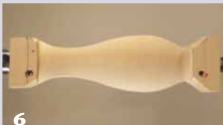
6 The workpiece is reshaped between centers.
