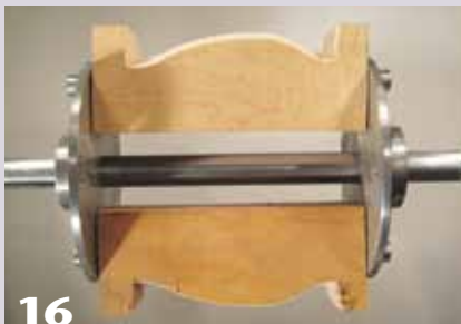
16 The first face of the workpieces has been turned and the pieces are ready for remounting.
