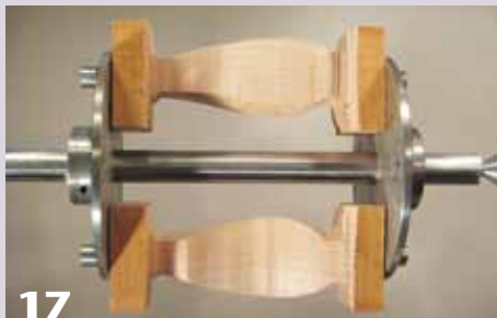
17 The two workpieces mounted to the jig after the fourth faces have been turned.
