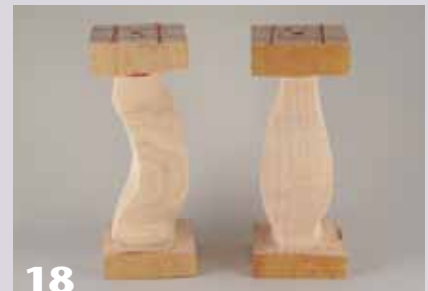
18 The two workpieces look like this after being dismantled from the jig. The two (identical) workpieces are rotated to show the different profiles.
