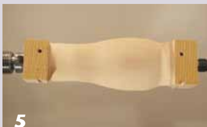
5 One of the workpieces has been remounted and is ready for turning between centers. Notice that the unturned ends have been trimmed.
