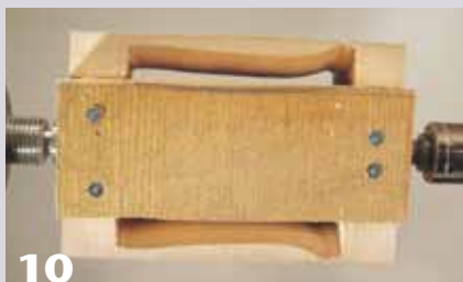
Photos 8 – 11 show a similar process, only with a 3" × 3" (75mm × 75mm) carrier in the middle. The pieces are thermed on the two broad faces.
