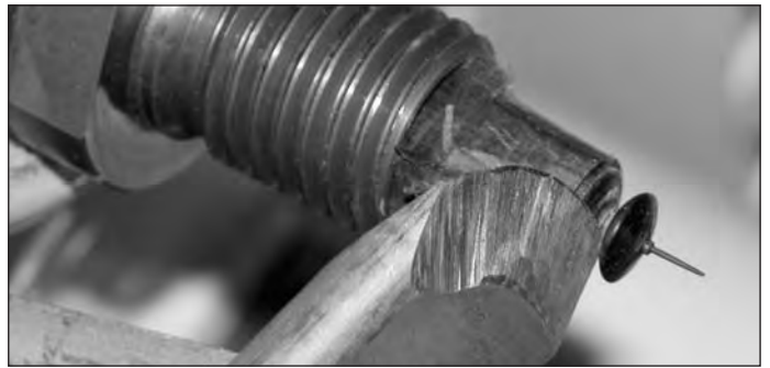
When working small diameter miniatures, you really can raise the speed to fairly high levels. However, I was getting clean cuts on this \frac{3}{8} " piece at speeds easily below 1,000 rpm.
