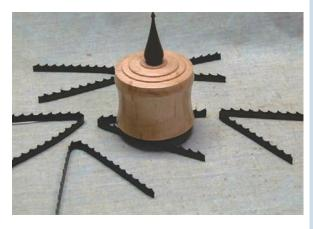
After applying finish to a woodturning, the item has to be placed somewhere to dry on something with minimal surface contact. I have made drying stand from dowels, nails, wires, and similar objects, but with mixed results and satisfaction. Items often did not balance correctly, or there was too much surface contact, or whatever I had set up was not the proper size for what I needed. In addition, any system I used took up too much storage space.
