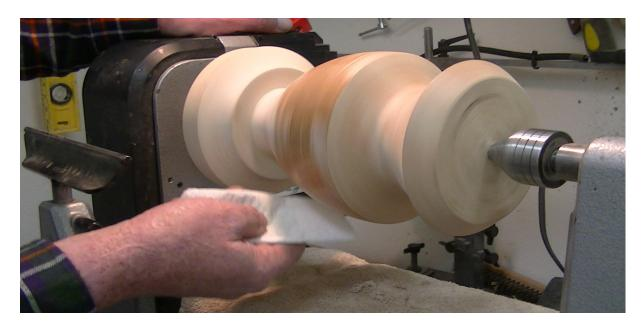
Now that the CA glue has been applied and smoothed, I will allow the project continue spinning at low speed for a short time to prevent the finish from running toward the lower part of the surface. If you speed it up too much the CA glue will tend to not even out on the surface because of the centrifugal force created by the spinning. (This can result in more sanding between coats to achieve a smooth surface.)
