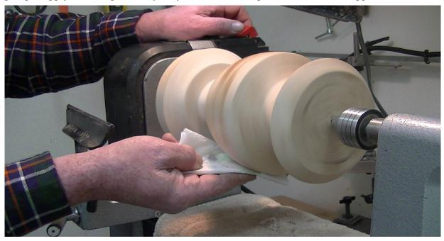
Now I just hold the applicator to the spinning project and allow the CA glue to evenly coat the surface. If you are using a 300cps CA glue, as I do, you will have plenty of working time to smooth it out as you go.
