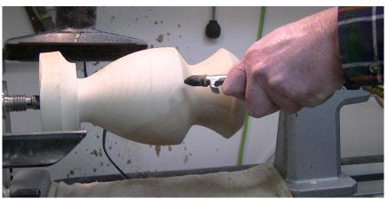
At this point I place a towel on the lathe bed directly under the project to protect the bed from any CA glue that might spin off of the project.
