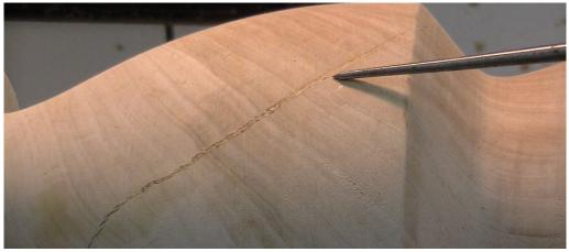
If you try to apply too much CA glue to fill a crack, the CA glue will form a skin which cures on the surface while the CA glue beneath it remains in a liquid state that requires more time to cure. The results are likely be that the liquid CA glue under the cured skin will spin out under the pressure of centrifugal force that is created when you restart the lathe. I have found that it is best to mix sawdust or other material(s) with the CA glue when using it to fill cracks.
