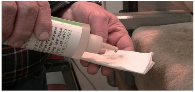
With the lathe spinning at its slowest speed I apply some CA glue to the paper towel. Remember, you are going to apply the CA glue thinly, so you don't need to put too much on the applicator.
